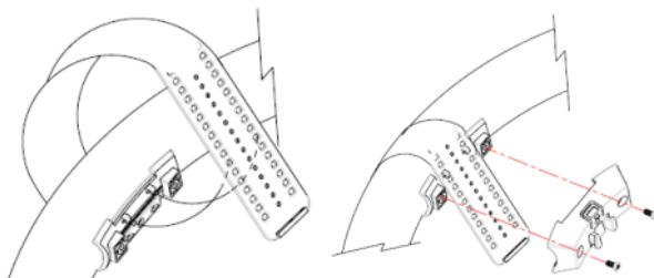
Step 3. Insert the prepared remote in the direction of the down arrow. If you detach the remote, hold down remove hook and pull it upwards to remove it.
