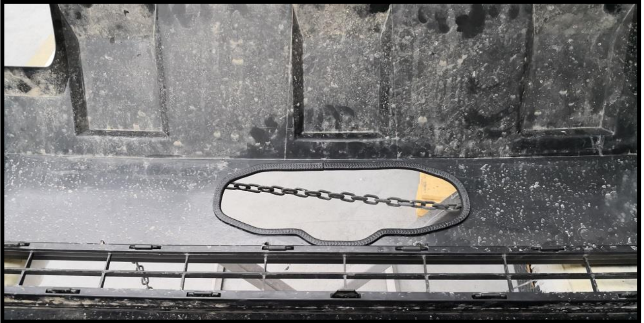
Dopasowanie plastiku + mocowanie kedry. Adaptation of the plastic + fixing of the rubber cover.
