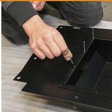
Put the rivets into the pre-drilled holes.
