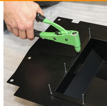
Use a riveter to fasten the rivets.
