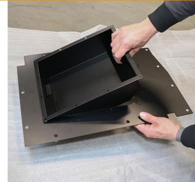
Put the locker inside the sheet. Make sure the angled side faces the center of the vehicle.
