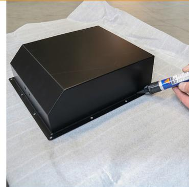
Apply sealant thinly on the entire underside of the locker's rim.
