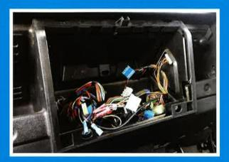
When the switches, headlamp levelling switch, power socket and radio mounting cage have all been installed, you are now ready to install the MUD Td5 Double DIN Console back into your vehicle. Replacement of the MUD Td5 Double DIN Console is the exact reversal of removal.
