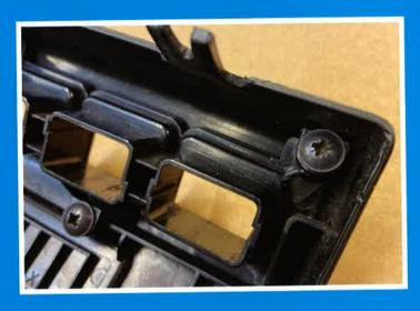
If you have a headlamp levelling switch installed, pull off the rotary knob to reveal the securing nut underneath. Undo the nut to release the levelling switch from the console.
