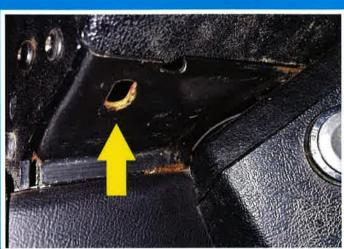
Remove the heater control fixings x 2 (yellow) and loosen the lower fixing circled (red).
