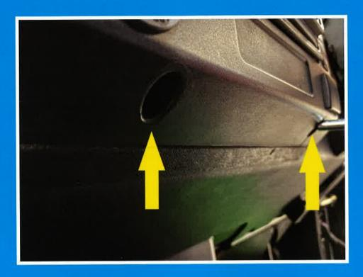
Loosen the three screws across the top of the radio console. You DO NOT need to remove these screws completely since you'll notice the three plastic locating tabs on the top of the console are slotted. The fixing screws clamp down on these slotted tabs. With the screws loosened you can now pull the console clear of the dashboard and begin to disconnect the radio, switch connections etc.
