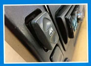
Remove the full width switch retainer housing from the back of the original radio console and transfer over to the MUD Td5 Double DIN Console. Secure to the Double DIN Console by reusing the original screw fixings. Refit the switches into the MUD Td5 Double DIN Console in their respective locations.
