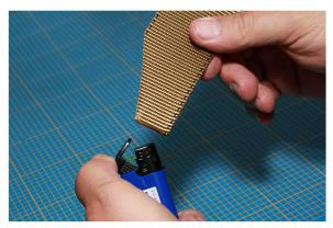
Please do this step outdoors: Flame the edges on both sides with the lighter until the ends of the fibres are sealed.
